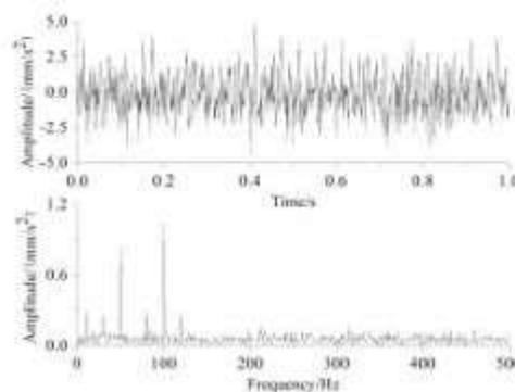
Fig.3 time domain and frequency domain waveform of single-channel mixed signal
